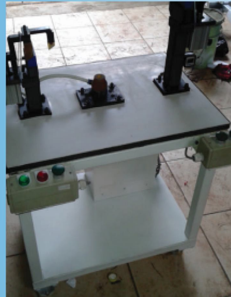
Equipment Leak Test Full Tank
