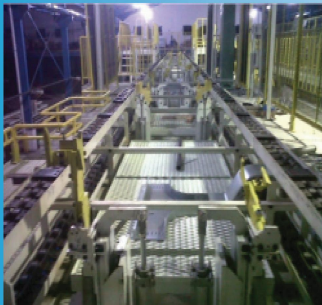
Equipment Process Under Body Locator
