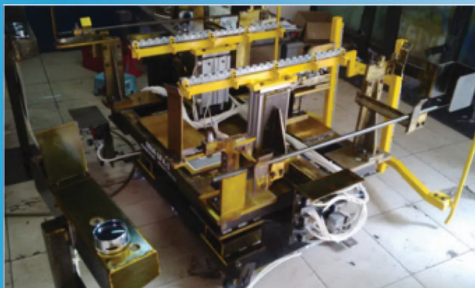
Welding Jig Fr Floor
